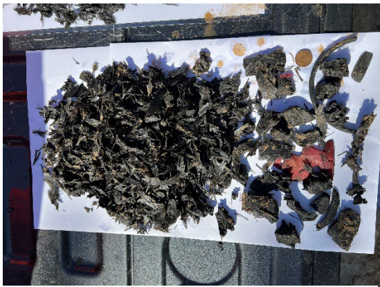
Figure 1: First ONEplug and remainder of debris from kill plug (seen in red)
