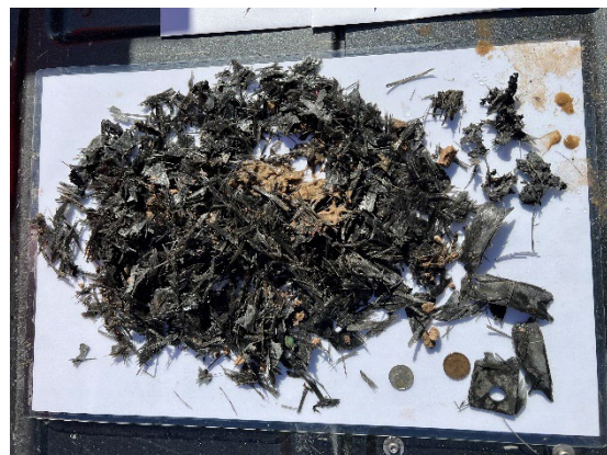
Figure 2: Debris from #2 and #3 ONEplug
