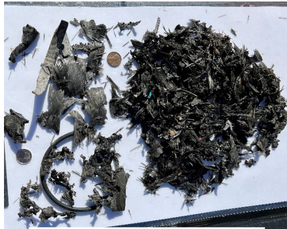
Figure 3: Debris from #4 and #5 ONEplug
